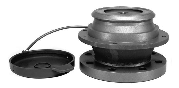
Eaton's Carter 4 inch adapters are made in accordance with API Bulletin 1584 to mate API 1584 compliant hydrant or bottom loading couplers. These adapters are furnished with flanges to mate 4 inch ANSI 150 lb. flat or raised faced flanges. Both ductile iron and aluminum materials are available. These adapters are designed to be used for bottom loading of a refueler, for connection to a hydrant system or for tank farm pumping system for test adapters.
